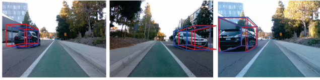
Figure 13: Predicted 3D bounding boxes using only radar (red) along with ground truth boxes (blue). The 3D IoUs of predictions are 0.52, 0.43 & 0.83 respectively. Radars can be used as a standalone sensor for object detection despite sparsity and low resolution.
